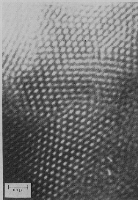
Figure 10. Electron micrograph of bSBS-2 block copolymer. Domain diameter equal to 235 ( \pm 15 ) Å. The nearest interdomain distance is 435 Å and the next nearest interdomain distance is 745 Å.
